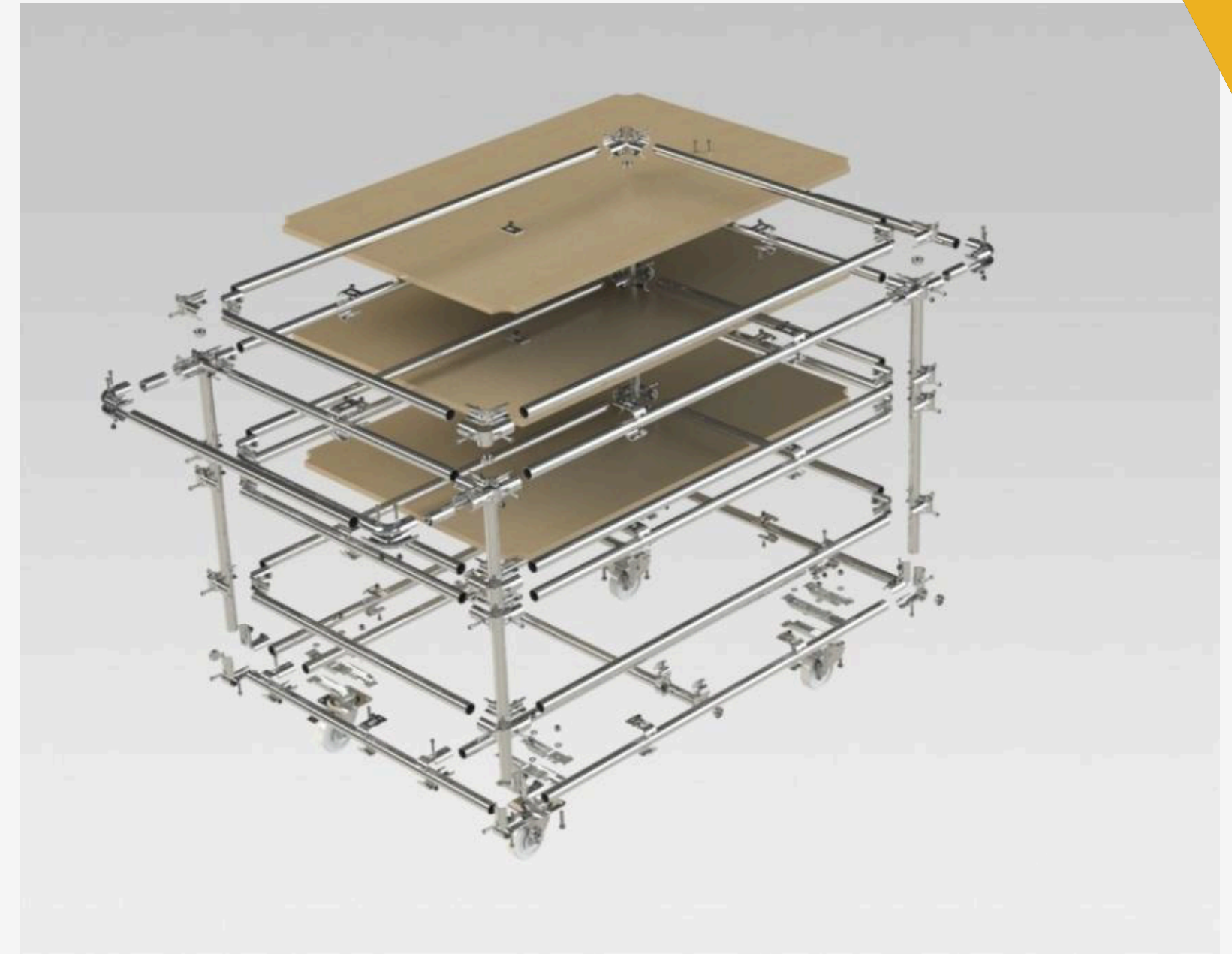
Exploded view of a transport trolley
